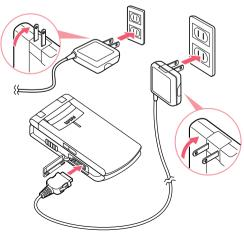
Check the shape of the connectors to ensure they are aligned correctly when you connect.
