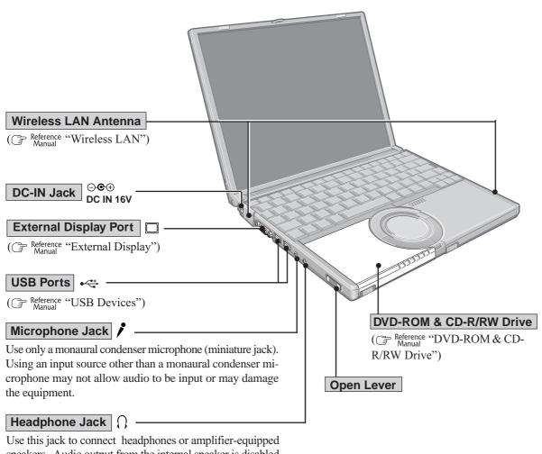
speakers. Audio output from the internal speaker is disabled when headphones or external speakers are connected.
