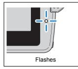
Flashes while the camera is accessing the memory card, such as recording images to memory card or reading files. Do not open the card/battery cover or remove the memory card while the LED is flashing as this could cause data corruption or, in some cases, camera damage.
