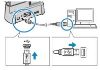
**Important** Check the sizes of the USB connectors. Plug the small connector into the USB cradle and the large connector into the USB port on your Macintosh.
