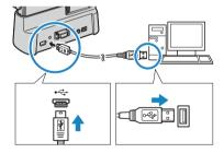
• Important Check the sizes of the USB connectors. Plug the small connector into the USB cradle and the large connector into the USB port on your PC.
