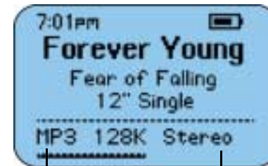
Track Information: Codec, Encoding Bitrate and Stereo/Mono Mode Indicator (from track ID3 tag information)
