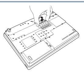
Sample inserting the memory module into the slot
