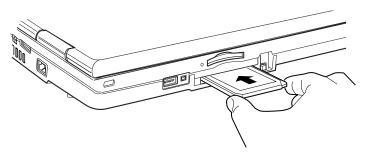
Sample inserting a PC Card
