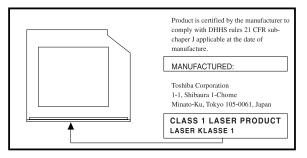
**ACAUTION** This appliance contains a laser system and is classified as a "CLASS 1 LASER PRODUCT." To use this model properly, read the user's guide carefully and keep it for your future reference. In case of any trouble with this model, please contact your nearest "AUTHORIZED service station." To prevent direct exposure to the laser beam, do not try to open the enclosure.
