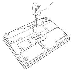
Sample removing the memory module slot cover
