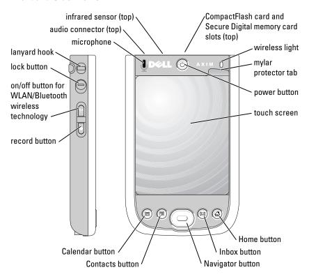
**INFRARED SENSOR** — Transfer files from your device to another infrared-compatible device without using any cable connection.
