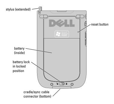
**BATTERY LOCK** — Use this switch to release and remove the main battery. See "Installing and Removing the Battery" on page 42.
