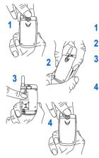
Switch off your phone and disconnect the charger. The SIM card is inserted beneath the phone's battery.
