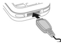
The battery is not fully charged when delivered. Plug the charger cable into the bot-
