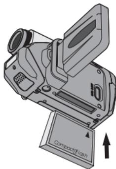
To remove the card, first make sure that the power is off. Then open the LCD panel, and push the card eject button to pop out the card or microdrive.
