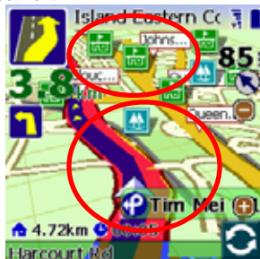
《Figure4-2-1b》 Simulating by standard speed 85km/h. Click on the center to enter setting. Click on upper row to enter search options.
