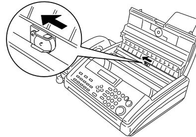
5. Install the paper roll. (Hold the roll so that it rolls away from you when pulled upwards.)
