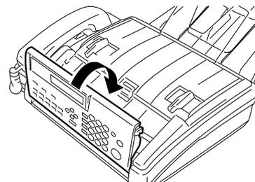
**NOTE:** If you hear an unusual noise when you are closing the operation panel, check the green levers have been pulled down to the bottom correctly.
