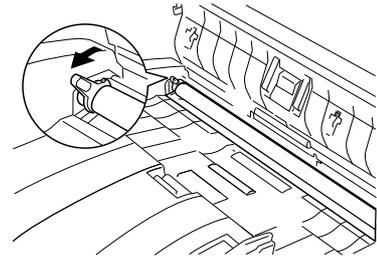
4-5) Make sure the levers are pulled down. Close the operation panel until it audibly locks into place.
