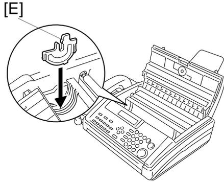
2-4) Insert the rod into the paper roll as shown, then set the roll into the machine (hold the roll in a direction so that it rolls away from you when the leading edge is pulled upward).
