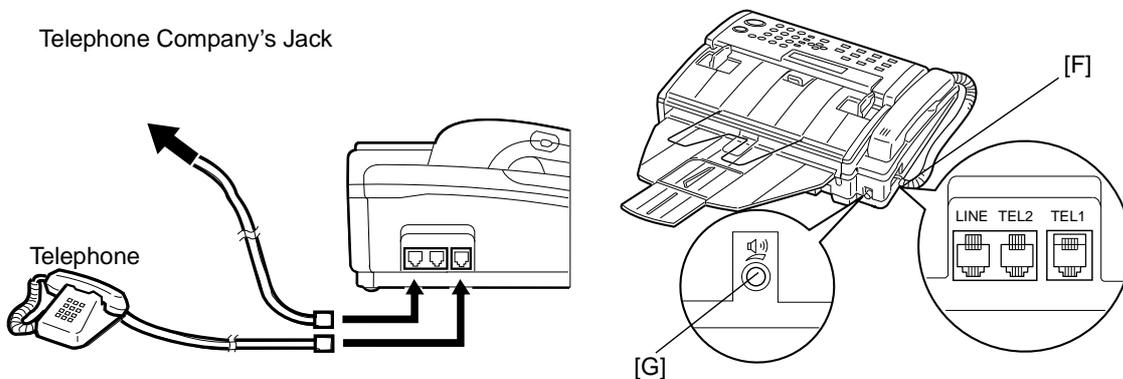
4. Adjust the speaker volume using the dial [G] at the back of the machine.
