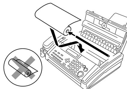
6. Pull out the leading edge until you can see it and feed the paper between the roller and the cover until it appears outside the back of the machine.
