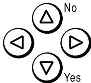
On the operation panel, there are four buttons (▲▼◀▶). They show the directions up, down, left and right. These are the scroll keys. They are often used in the operating procedures to gain access to various features. For example, if you see "Press the ▶ key" in the manual, you are being asked to press the right-pointing arrow of the scroll button. On this machine, the ▲ key also acts as the **No** key, the ▼ key is used as the **Yes** key.
