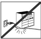
Do not place heavy items on the power cord. Power cord damage can lead to damage of the equipment (fire hazard) and can cause electric shock.
