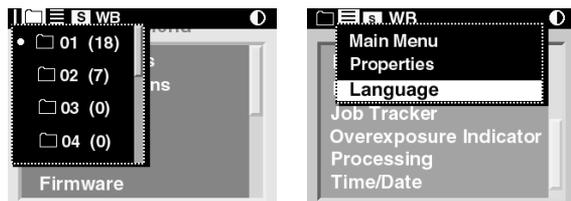
2 Press the top or bottom of the Four-way switch to highlight a menu option.
