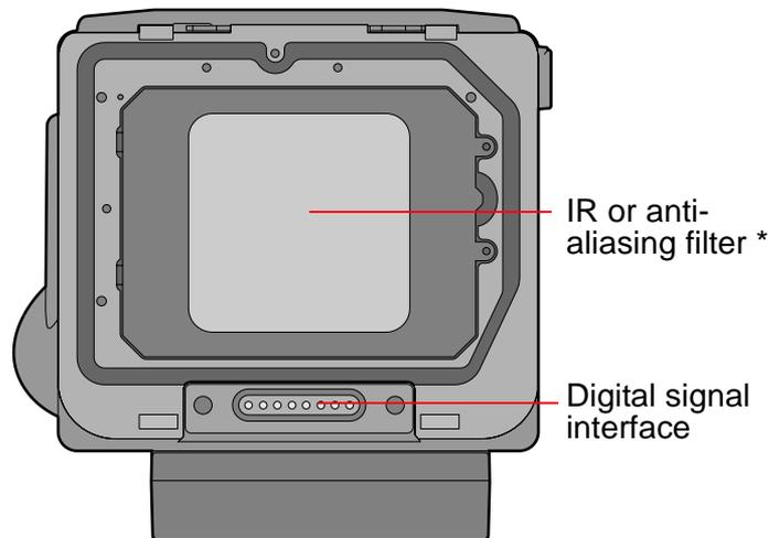
\* For your images to be sharp and in focus, you must use either an IR filter or an anti-aliasing filter.
