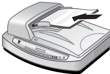
load paper and center in the tray
