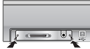
tighten the two mounting screws
