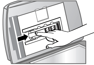
insert the negative light-shield
