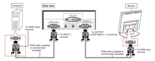
You can display computer images on a monitor using the RGB cable.
