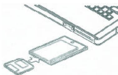
If you are using a PC card reader, first insert the SD card into a PC card adapter (optional), and then insert the PC card adapter into the computer's PC card reader.
