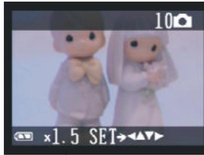
If an image is magnified, the ratio indicator will display on the left down side (next to the Battery Indicator) of the LCD screen.
