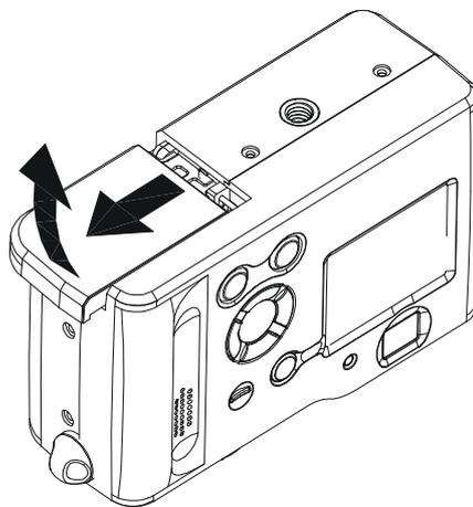
3. Check inscription on battery chamber for correct negative/positive installation.
