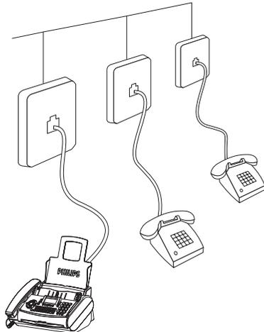
⚠ If you connect additional devices to separate sockets (e. g. in separate rooms) your fax switch cannot control them (which means that your machine behaves like any ordinary machine). For this reason e. g. call transfer is not possible. Therefore we recommend you to connect your additional devices to the same socket.
