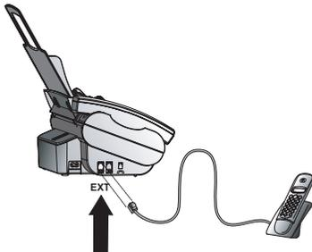
⚠ Connecting additional devices to the same socket ensures you the optimal functioning of your fax switch (e. g. call transfer). Your fax machine can control the additional devices.
