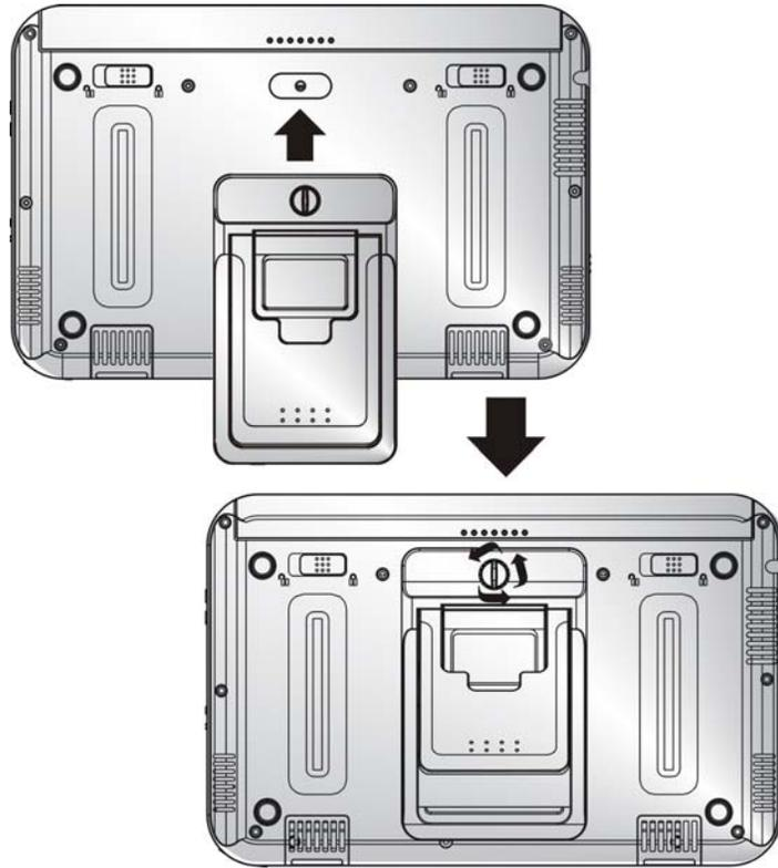
There are two ways to use the stand; the upper portion will support your system at a lower angle (20°) when you are operating on the table.
