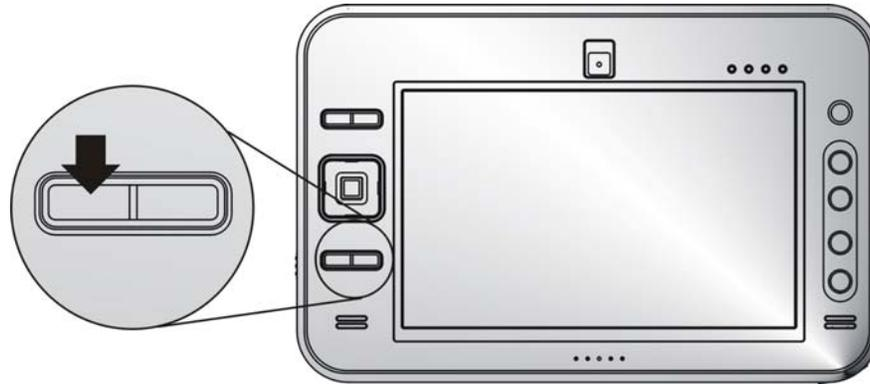
Press the Origami button to display the Origami application as shown on the top illustration.
