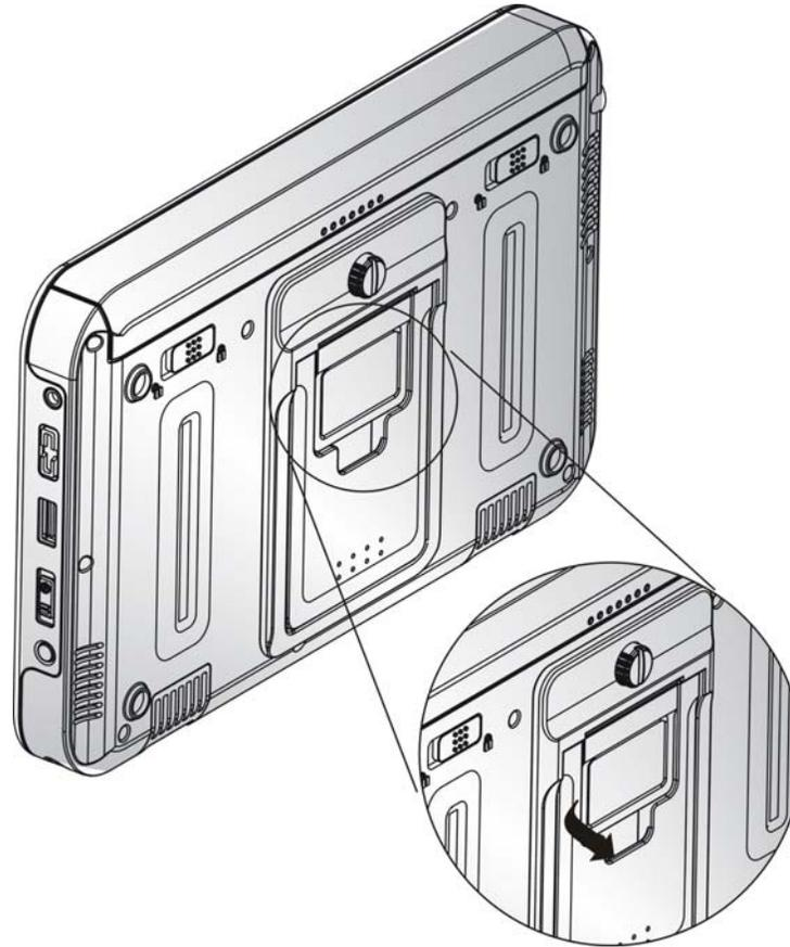
The lower portion will support your system at a higher angle (80°) when you are operating for a much clearer view.
