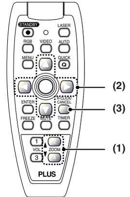
**(2) Pressing the SELECT (▲▼◀▶) buttons on the remote control at the time of the zoom operation will cause the display position to move.**
