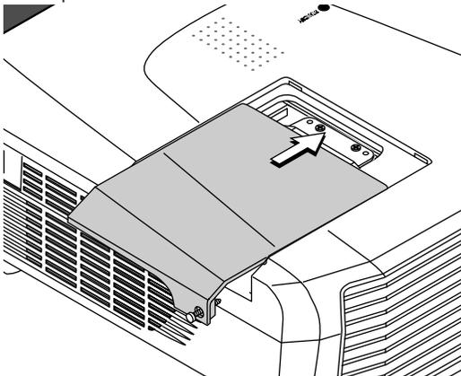
(2) Turn the lamp cover's screw clockwise to tighten it.
