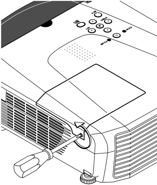
(2) Open the lamp cover a little, then pull it in the direction of the arrow and remove it.
