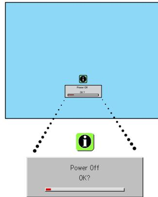
The STANDBY indicator changes to blinking amber and lights a steady amber after about 90 seconds (when the unit enters the standby mode).
