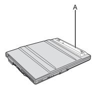
At the time of purchase, the stylus (included) is not attached to the stylus holder (A). The tether prevents the stylus from falling accidentally. It can be attached to the stylus holder.
