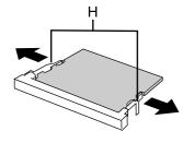
① Gently open the left and right hooks (H). The RAM module will be raised at an angle.
