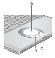
Use the touch pad to move the cursor on the screen and perform computer operations.
