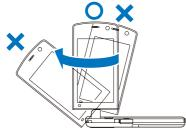
• When you rotate the display, be careful not to touch the corner of the display to the keys or body. Moreover, you cannot rotate the display counterclockwise or over 180 degrees. Forcing to rotate the display may cause damage or malfunction.
