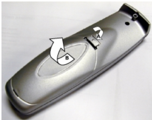
Image 3-6 Battery cover unlock
