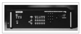
An optional RCVDS05 makes it possible to connect up to 20 sources to the projector. When RCVDS's are linked via the expansion module, even 90 inputs can be connected to the projector.
