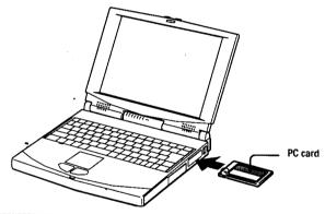
Do not force a card into the slot. It may damage the connector pins.
