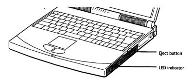
If you have difficulty removing a diskette from the floppy disk drive, remove the floppy disk drive from the drive bay.
