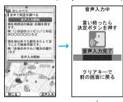
The confirmation display appears after your voice is recognized. When the recognition is wrong, select "音声再入力(Re-input voice)".
