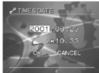
Press the ◀ or ▶ button to select the item to set, and press the ▲ or ▼ button to set the value for each item. Press the **ENTER** button when **OK** is selected, date and time data is updated.
