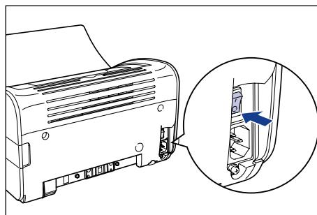
**2 将提供的电源线稳固地插入电源插孔中。**
