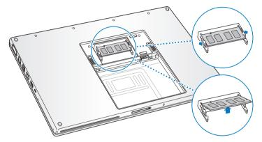
4 Insert the memory card at a 25-degree angle. Line up the notch in the card with the small tab in the memory slot and slide the card into the slot until the gold edge is almost invisible. Then firmly push the memory card into the memory slot. You might feel some resistance.
