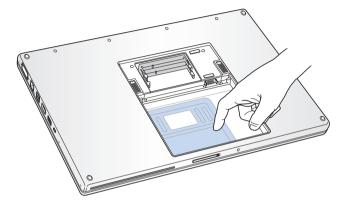
3 If you need to remove a memory card that's already installed in the slot, spread the tabs in the slot away from the notches in the memory card. The card should pop up slightly. Lift the memory card to a 25-degree angle and then gently slide the card out of the memory slot.
