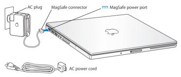
To extend the reach of your power adapter, first pull the AC plug up to remove it from the adapter. Attach the included AC power cord to the adapter, making sure it is seated firmly. Plug the other end into a power outlet. The AC power cord provides a grounded connection.
