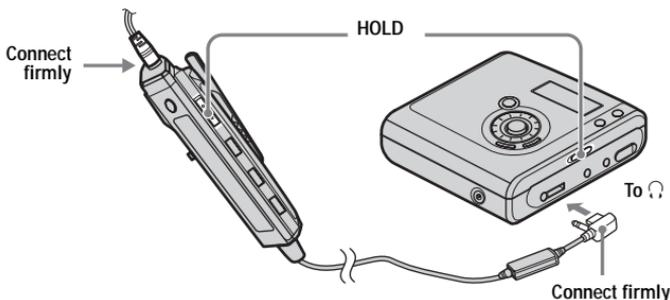
2 Slide HOLD to the opposite direction of the arrow ( $\rightarrow$ ) on the recorder or the remote control to unlock the controls.
