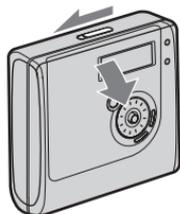
2 Insert a disc with the label side facing front, and press the lid down to close.
