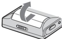
2 Insert a LR6 (size AA) alkaline dry battery  $\ominus$  end first.
