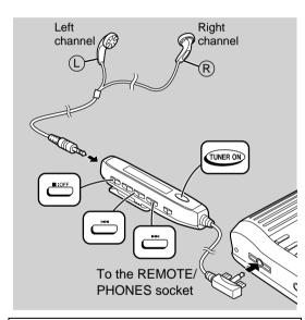
In the tuner mode, you can use the remote control. Buttons on the main unit are disabled (except the ■:OFF, ▶II and REC buttons).
