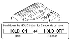
If the battery is inserted or the AC adaptor is connected, you can set this function even when the power is turned
