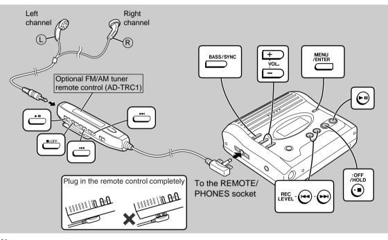
To operate without the FM/AM tuner remote control, connect earphones to the REMOTE/PHONES socket.
