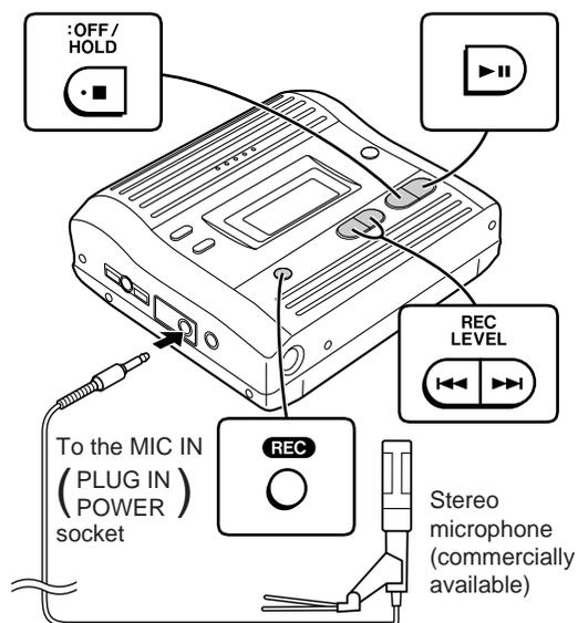
**1** Connect a stereo microphone to the MIC IN socket.
