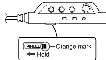
Move the HOLD switch to the safety position (direction indicated by the arrow).
