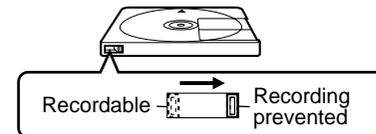
To add a recording to such a MiniDisc, slide the accidental erase prevention tab back to its original position.
