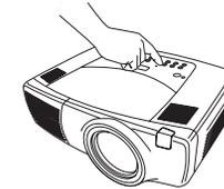
If the image is not on the screen or viewing area, adjust it by pressing the lens shift button on the keypad.
