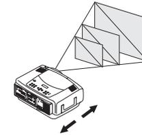
Adjust the zoom or focus by pressing the power **Zoom** or power **Focus** buttons on the keypad until the desired image size and focus are produced.
