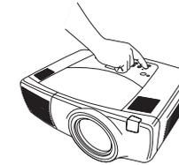
Adjust the volume on the keypad or remote.
