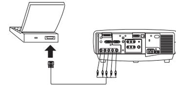
You can control the projector from an LCD control panel, touch screen, or other control device or computer by connecting an RS-232 cable to the projector's **Serial** connector. Specific RS-232 commands can be found in the Service and Support section of our website and in this User's Guide's Appendix.
