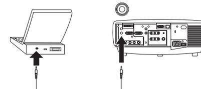
If you are using a desktop computer and want to see the image on your computer screen as well as on the projection screen, plug the monitor cable to the **Monitor out** connector on the projector.
