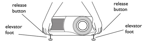
Position the projector the desired distance from the screen at a 90 degree angle (perpendicular) to the screen.
