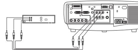
You can also connect to your video device using a BNC cable. Connect the BNC connectors of the BNC cable to the appropriate **Computer 3** connectors on the projector. Connect the other end to the video port on your video device. Use the A/V cable's audio connectors as described on the previous page (the yellow connectors on the A/V cable are not used).
