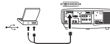
If your projector cannot receive the remote's signal due to IR interference, you can connect directly to the projector via a remote cable. To do so, plug the remote cable into the wired remote connector on the projector. Plug the other end into the connector on the remote,
