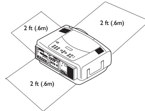
Do not place objects in the areas along the left, back and front sides of the projector. For ceiling mount applications, this area should be 5 feet (1.5m).
