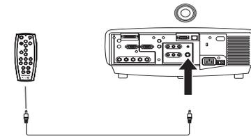
To have sound with your presentation, connect the audio cable to your computer and to the corresponding computer **Audio In** connector on the projector.
