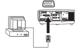
You can also connect to your computer using a BNC cable. Connect the BNC connectors on the BNC cable to the appropriate **Computer 3** connectors on the projector. Connect the other end to the video port on your computer. If you are using a desktop computer, you first need to disconnect the monitor cable from the computer's video port. When all 5 BNCs are connected, the projector handles separate synchs on H and V.
