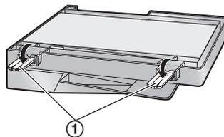
3. Insert the hinges (①) into the slots (②) on the unit.
