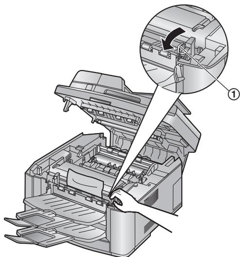
2. Remove the jammed paper (①) carefully by pulling it upwards.
