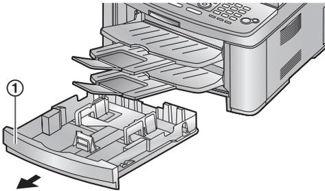
2 Pinch the front side of the recording paper guide (①), then slide it to match the paper size mark.
