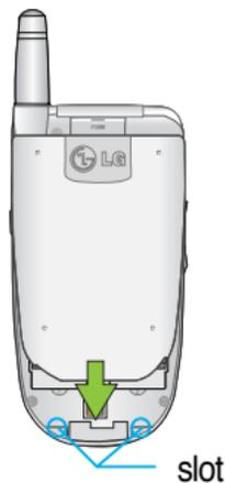
To install the battery into the phone, insert the battery into the battery slot at a slight angle and press the top of the battery until the battery clicks and locks into place.
