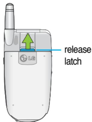
To remove the battery from the phone, push the battery release latch and then pull out the battery from the phone.
