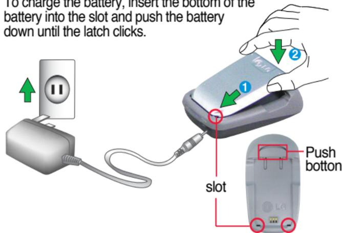
To remove the battery, press Push button
