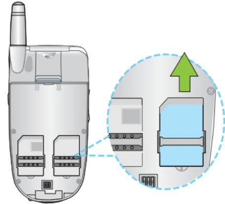
To take out the card from the phone, push the lock device to the up side and then pull out the card from the phone.
