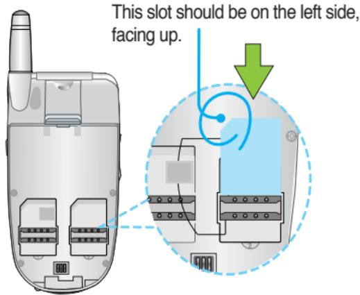
To insert the card into the phone, push the card into the bottom side until it click and locks into place.
