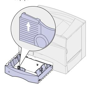
Note: Do not exceed the maximum stack height. Overfilling the tray may cause jams.
