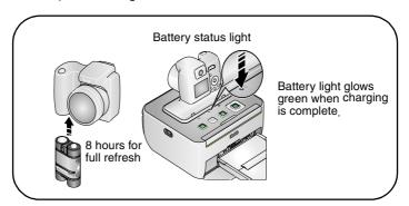
NOTE: If you are getting fewer than 20 pictures per charge, you may need to refresh the battery. The refresh cycle completely discharges the battery, then fully charges it. See Extending battery life, page 60.
