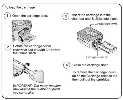
**IMPORTANT**: Remove the cartridge when the cartridge light glows red (see page 49).
