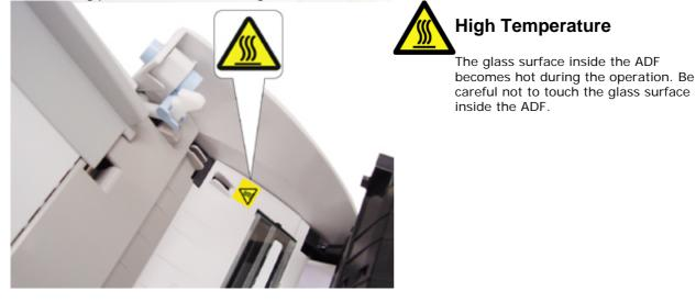
ATTENTION Do NOT remove from the scanner, stain or scratch the warning labels.
