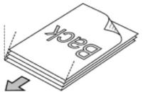
4. Load the documents into the ADF chute, as shown in the picture.
