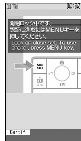
Stand-by display appearing when Lock on close is activated from a screen except stand-by display
