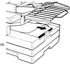
Press the printer cover release button and open your fax machine's printer cover.
