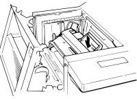
**6** Close the printer cover. Push down on the cover to lock it into position.
