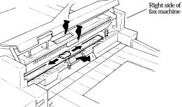
Gently close the scanner cover, making sure both sides are snapped down securely.
