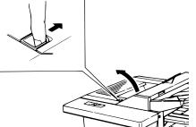
**5** Gently close the printer cover, pressing firmly on both sides of the printer cover until you hear it click.
