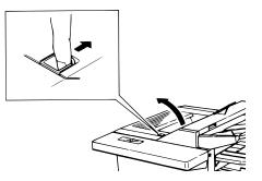
**2** Gently pull the jammed printout *up and out.* The printout may be jammed either within the fax (*left*, below), or in the output tray (*right*, below).
