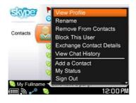
2 Press △/▽ to select "Exchange Contact Details," and then press the center button.
