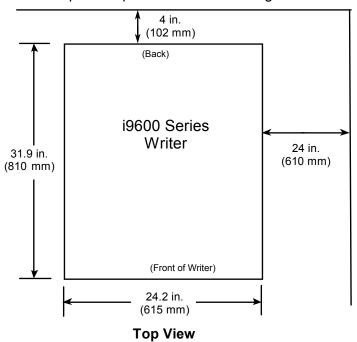
The Writer is on casters so it can be moved to reach the main power switch located in the back of the unit. All operator procedures are accessible from the front of the unit.
