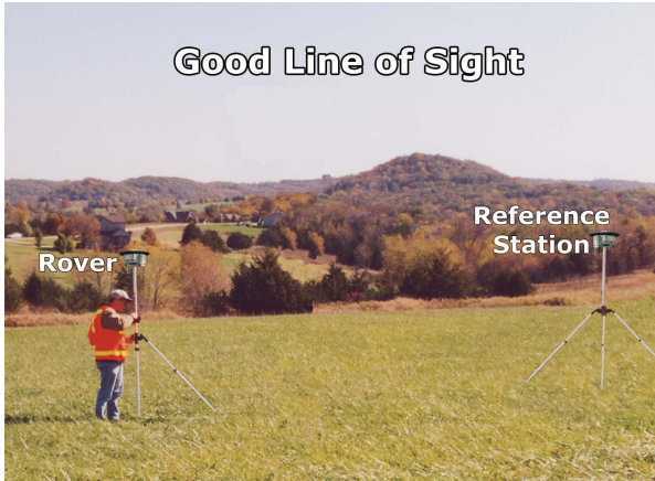
Figure 8: Good Line of Sight RTK setup
