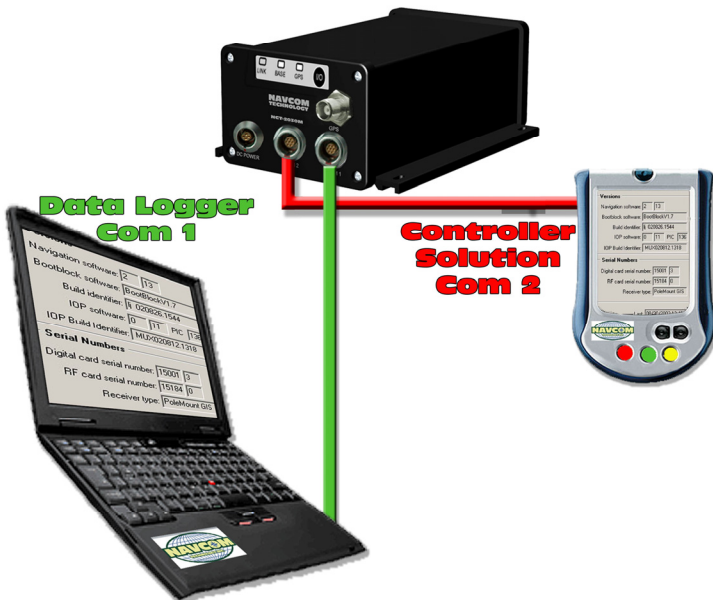
Figure 8: Communication Port Connections
