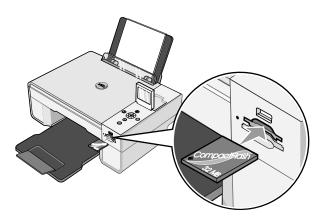
**NOTE:** Do not remove the card while it is being read. Data corruption can occur.
