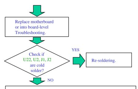
One of the following parts on the mother-board may be defective, use an oscilloscope to check the following signal or replace the parts one at a time and test after each replacement.
