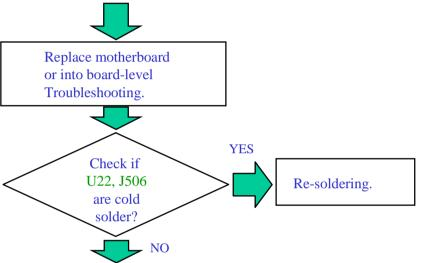
One of the following parts on the mother-board may be defective, use an oscilloscope to check the following signal or replace the parts one at a time and test after each replacement.
