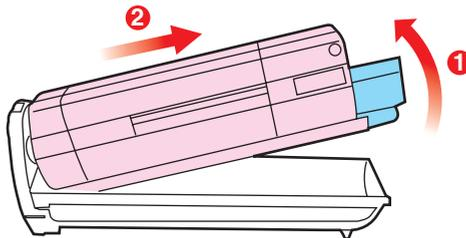
7. Take the new image drum cartridge out of its packaging and place it on the piece of paper where the old cartridge was placed. Keep it the same way round as the old unit. Pack the old cartridge inside the packaging material for disposal.
