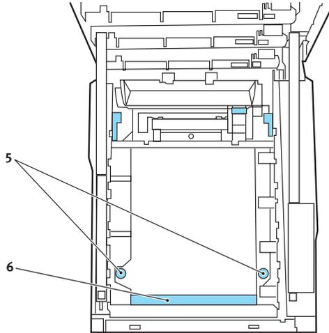
5. Turn the two fasteners 90° to the left. This will release the belt from the printer chassis.
