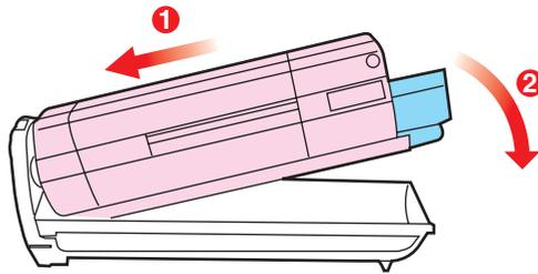
9. Push the coloured release lever (1) away from you to lock the toner cartridge onto the new image drum unit and release toner into it.
