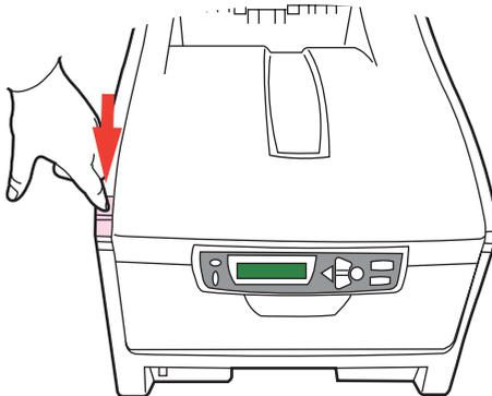
2. Identify the fuser handle (1) on the top of the fuser unit.
