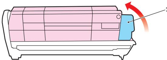
10. Holding the complete assembly by its top centre, lower it into place in the machine, locating the pegs at each end into their slots in the sides of the printer cavity.
