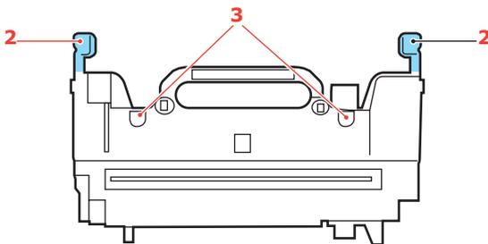
7. Lower the fuser into the machine, locating the two lugs (3) into their slots in the metal partition which separates the fuser area from the image drums.
