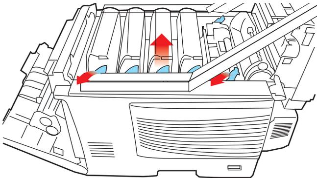
5. Lift the edge of the side cover slightly at the two points shown, and pull the cover away from the printer at the top. Lift the cover slightly to detach it from the printer. Place it safely to one side.
