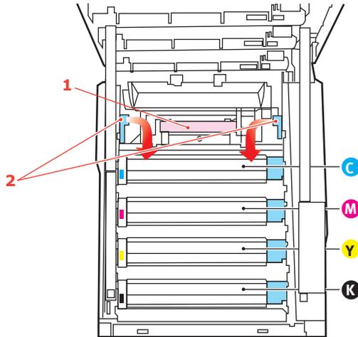
3. Pull the two fuser retaining levers (2) towards the front of the machine so that they are fully upright.
