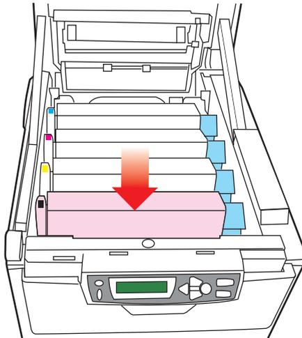
9. Lower the top cover but do not press down to latch it closed yet. This will protect the drums from excessive exposure to room lighting while you check the remaining areas for jammed sheets.
