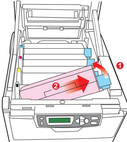
5. Put the cartridge down gently onto a piece of paper to prevent toner from marking your furniture and to avoid damaging the green drum surface.
