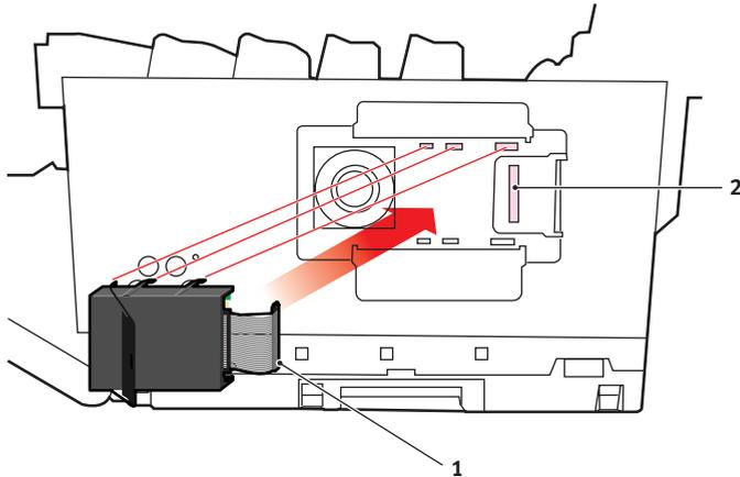
7. With the component side of the disk unit facing the printer, and the connector cable towards the rear, lift the disk unit handle away from the disk body.
