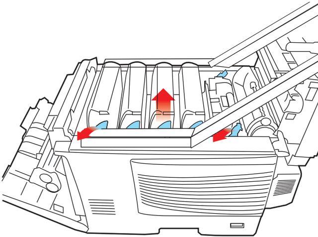
5. Lift the edge of the side cover slightly at the two points shown, and pull the cover away from the printer at the top. Lift the cover slightly to detach it from the machine. Place it safely to one side.
