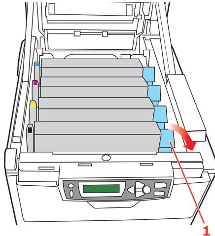
4. Lift the right-hand end of the cartridge and then draw the cartridge to the right to release the left-hand end as shown, and withdraw the toner cartridge from the machine.
