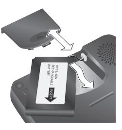
12V/24V power supply in your vehicle. The battery will then start to charge. It takes approximately 5 hours to fully charge the battery. The battery life without an external power source is approx. 3 hours depending on application and adjusted display brightness.
