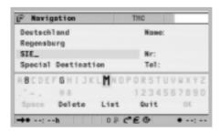
After input of the postal code, use "List" to display all corresponding town parts. Select the desired town and confirm with OK. The town name is also sufficient for a destination. The navigation system will then route you to the town border. A unique input is made with the postal code and the town name.
