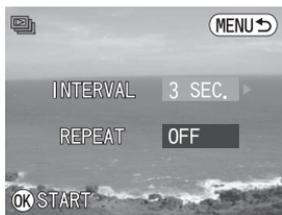
**2** Use **EV** button to select "INTERVAL" and use **EV** button to select the interval setting (1~10sec).
