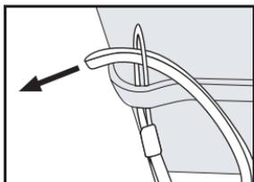
Insert the small loop of the wrist strap into the strap eyelet. Insert the long loop of the wrist strap into the small loop of the strap and then tighten it.
