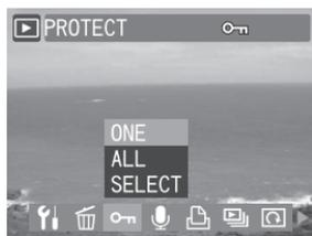
**3** A protected file is indicated by the mark. Follow step 1 and 2 again and then press OK button to remove the protection.
