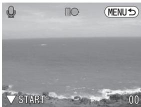
**3** Press **EV** button to start recording. When the voice memo recording starts, the indicator icon on the LCD monitor changes from (green) to (red). Press **EV** button again to stop recording and return to the previous menu.
