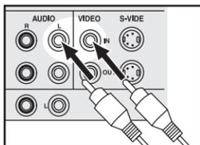
**2** Connect the A/V (Audio/Video) cable to the A/V inputs of the TV, and connect the A/V cable to the A/V connector of the camera.
