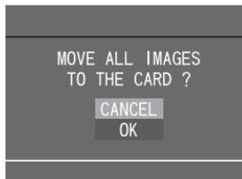
*Note: If the camera does not respond when you select the “Move Images to Card” function, either the memory card is not inserted or the card may be broken or locked.*
