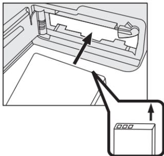
**2** Insert the battery. Please check whether the battery is inserted with the correct polarity (+/-).
