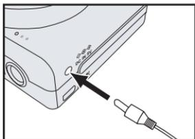
**1** Make sure that the camera is turned off. Plug the AC adapter connector into the “DC IN 5V” socket on the camera.
