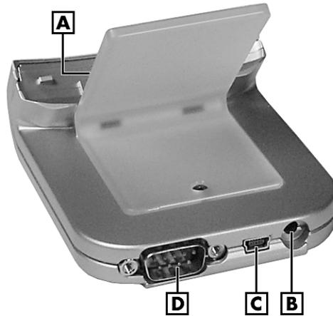
**A** – MobilePro Connector (on front)      **C** – USB PC Cable Connector
